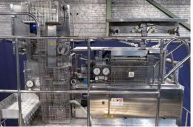
Aseptic form fill seal machine 1000ml Base line tetra carton Filler standard base line cartons 1.000ml, development controls 70V 45.334 production hours. Controls: TPMC 70V. With small standard Cleaning unit (CIP) Tetra model: SCU/4, machine nr 616054-0150 1 x roll feed trolley and a variety of spare parts. Part of top Fences Total dimensions 490 x 200 x 440 cm.
