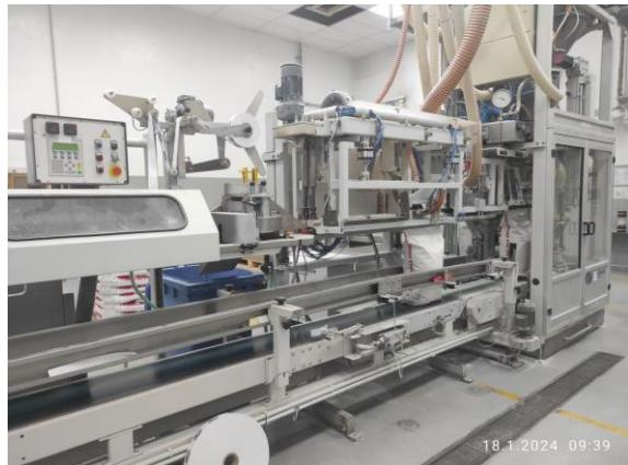
Milk powder bag filling line. Still in production till the end of February 2024. Line for filling (skimmed) milk powder in standard 25 kg bags. Including vacuum suction system to
