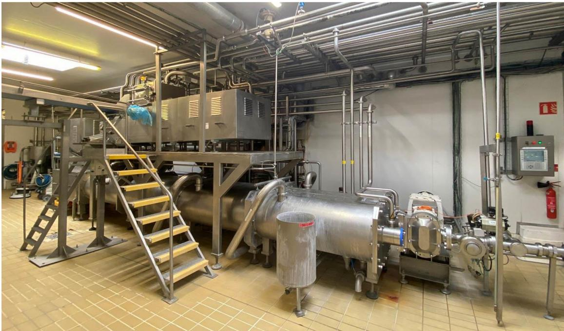
Deep frozen butter reworking machine for frozen 25 kg butter blocks. For reworking frozen butter blocks up to – 20°C. Excellent regulation of the butter temperature by control of the mechanical energy given to the product. Rationalizes the processing and packaging of the butter. Improving the quality by ensuring finest water dispersion resulting in an increased shell of life of the homogenized and packed butter.
