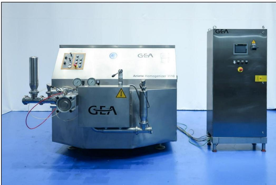
High pressure homogenizer. 2 stages with pneumatic pressure control. 3 Ceramic pistons, piston diameter: 55 mm and stroke: 100 mm. Stainless steel cladded with sound reducing material. Connections: 2 x 3" Din. Current motor power: 132 kW and maximum pressure in current configuration with this motor 450 bar. Freestanding control panel with Siemens
