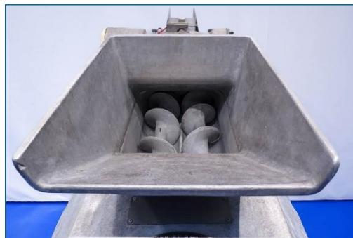
The Benhil Microfix rationalises the processing and packaging of cold store butter. The machine reduces the time it takes to defrost butter, it improves the quality of the butter by creating the finest water dispersion and improves the spreadability of the butter.
