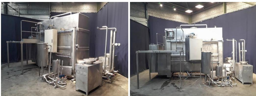
Closed butter silo. Buffer tank for butter before the butter is been packed. 2 augers to push the butter to the outfeed pumps. Including hot water preparation set with electric heating elements and circulation pump for CIP cleaning the silo. Including stainless steel stairs to the manhole to look inside the butter silo. Flange with 4 connections, 3 outfeed lobe pumps (make Simon Freres model: RS150), control panel (has to be renewed), piping and valves. Excluding CIP return pump.
