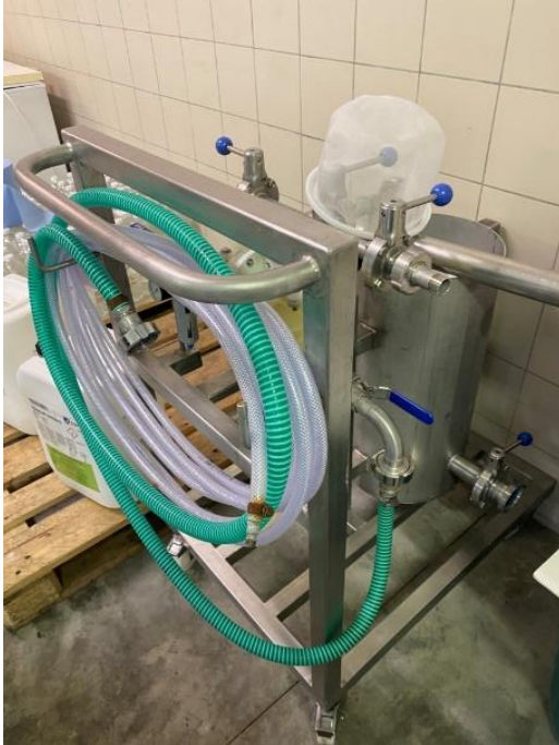
Brine filter system with pump and sieve
