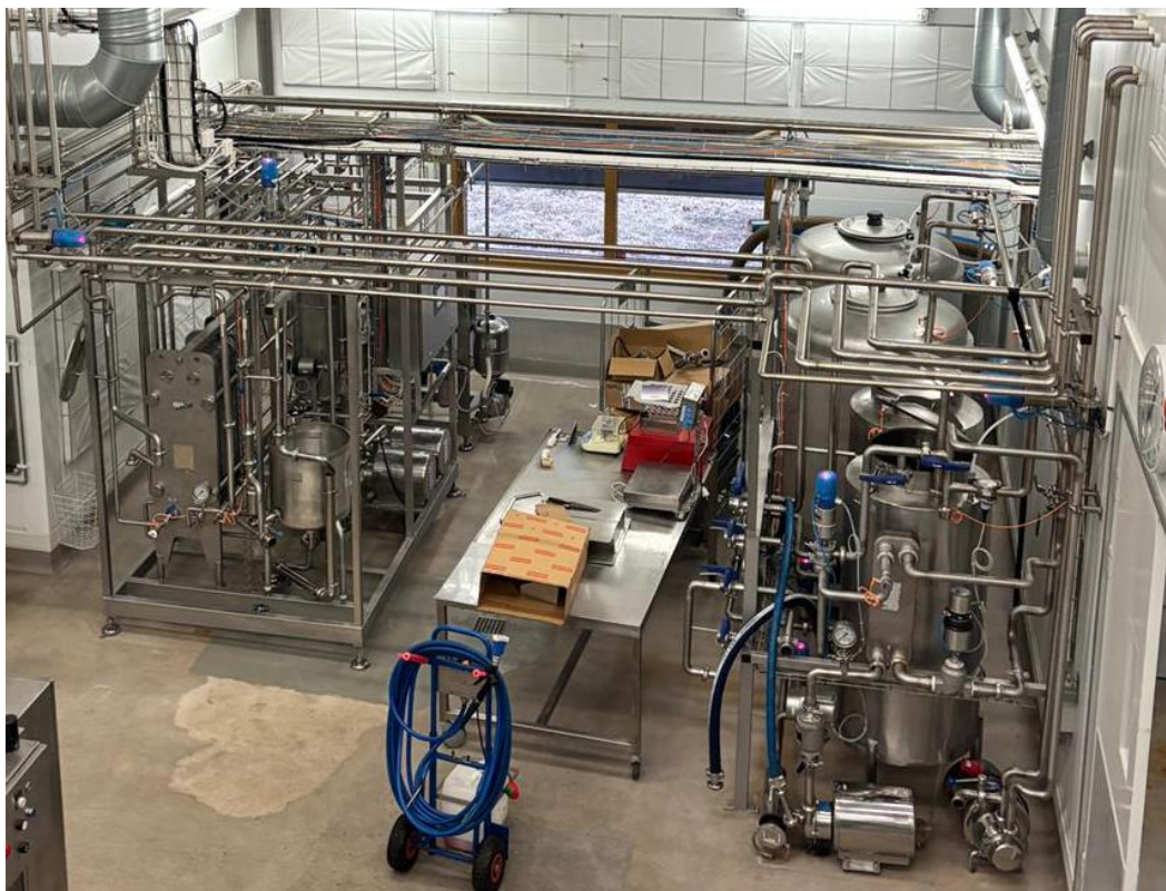
Overview picture: Pasteuriser and CIP system Total price – Pasteuriser and CIP unit: € 85.000
