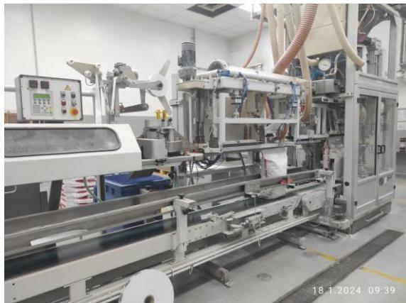
Milk powder bag filling line, was still in production until the end of February 2024. Line for filling (skimmed) milk powder in standard 25 kg bags. Including vacuum suction system to vacuumize the bags to increase the shelf life of the milk powder. Including vacuum filter.
