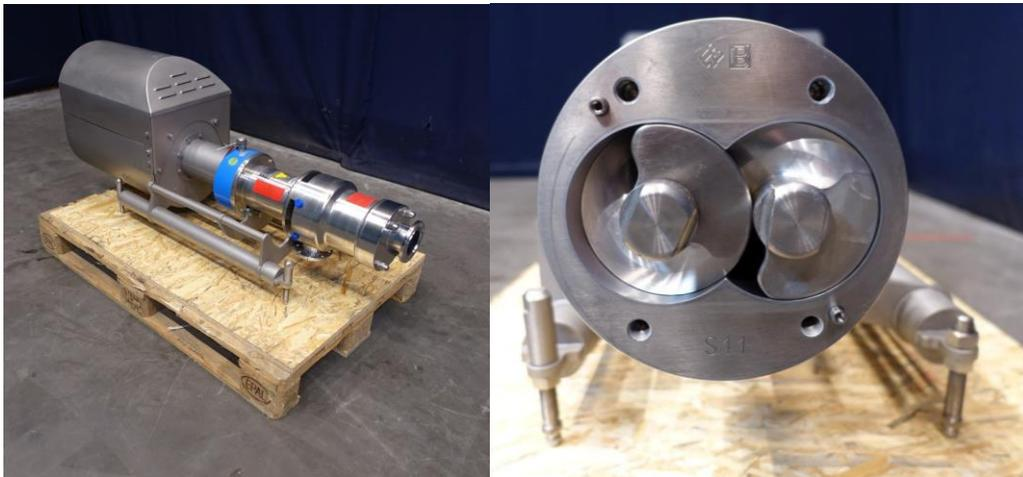
SLH Twin Screw Pumps are rotating positive displacement pumps, using two screws to convey the product along the screw axis. The contact-free intermeshing screws and the housing form closed chambers, constantly moving product from suction to discharge. By right turn of the drive shaft, the flow direction goes from the front axial to the mid top position. The pump can operate in the opposite direction as well. Reverse operation is possible to empty the suction piping from product before cleaning.
