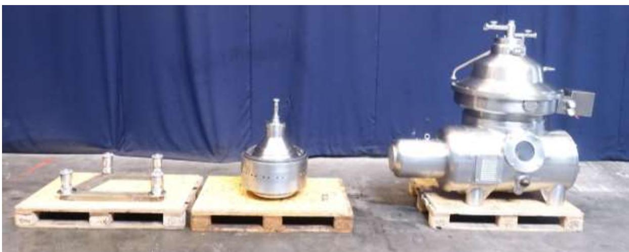
Bactofuge, self-cleaning. For bacteria spores removal. Including bowl, (bowl speed: 6.450 rpm) motor cover, base frame, and maneuvering water valves. Excluding: collecting tank, counter pressure valve, flow indicator and flow regulation valve for bactofugat, remix valve, set of tools and the controls. Previously used in a dairy school in Austria for tests only. Including operating manual and spare parts list in German.
